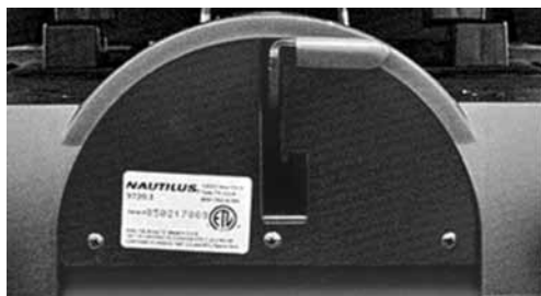
Lever in locked position for treadmill mode
