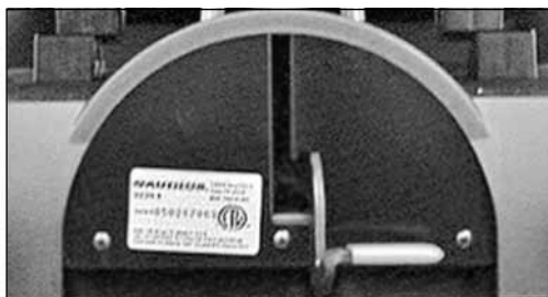
Lever in unlocked position for TreadClimber® mode
